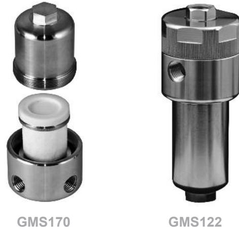
Guardian Membranes are also offered with integral coalescing pre-filters. A 50C grade element is mounted before the membrane to remove most liquids and solids, thus providing longer membrane life. This integral package minimizes dead volume, panel space, and leak points. The combo units accept the same membrane kits as our standard Guardian units. Part numbers are specified at the bottom of the attached chart.
